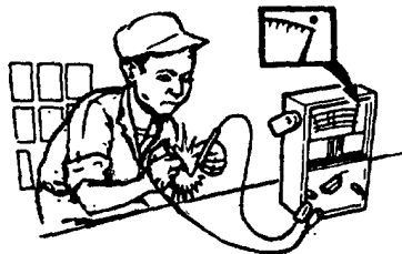
CHECK MULTIMETER FOR CONTINUITY
